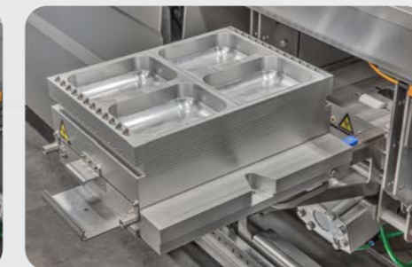
Quick tooling exchange for highest flexibility: our innovative quick exchange system from the side allows you to run different die sets.
